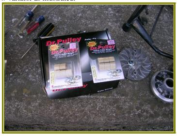
If you are using Dr. Pulley Sliding roller weights, orientation is critical or the variator will not function.
