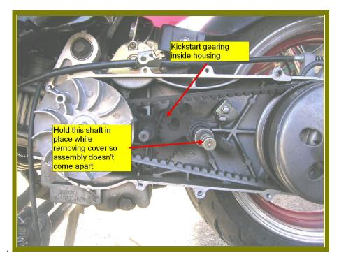
Note: On some scooters, the kick start gearing is attached to the inside of the transmission cover. In this case the shaft will stay attached to the cover when removed.
