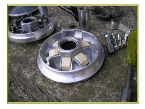
Install weights with proper orientation into the drive pulley. Place three nylon bushings onto ramp plate as illustrated and slide ramp plate onto drive pulley.
