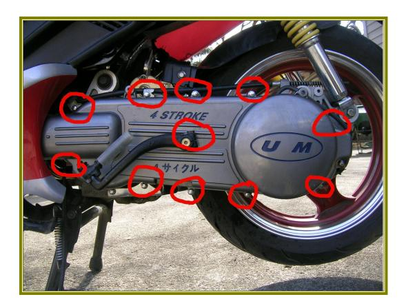
The screw attaching the kick start lever must be totally removed for the lever to slide off. The transmission cover bolts will be of different lengths, so make sure you make note of placement. Also make note of placement of any hose and cable guides held in place by these bolts.
