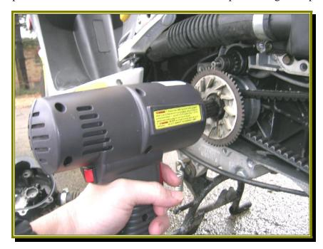
Remove the front fixed pulley.
