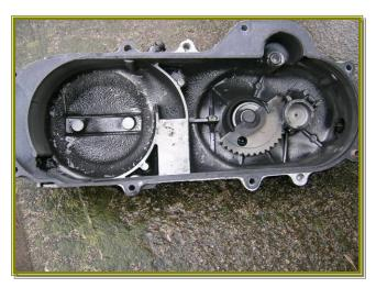
Use this opportunity to clean sludge from the cover and lube kick start gearing. In this illustration the kick start gearing is attached to the cover.
